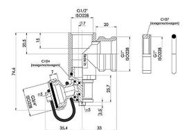
The end part with automatic air vent is supplied with Pintossi air vent art.507 which can be easily assembled using **PTM system**. In this version the drain valve can be moved in the preferred position.
